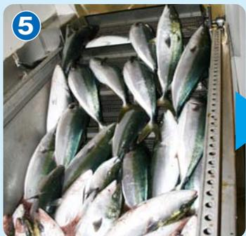
5 The fish are lifted by the Stainless Lift Conveyor and are carried from the fish receiving site to the sorting site.
