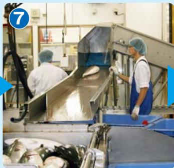
7 The round fish slide down to the sorting site by means of a shooter.
